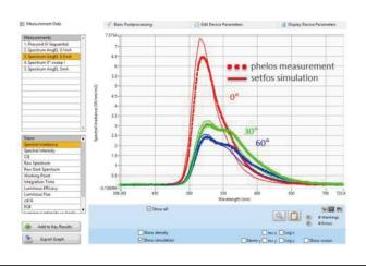
Setfos dipole emission and drift- diffusion model can be run directly from the Phelos control GUI.\*
